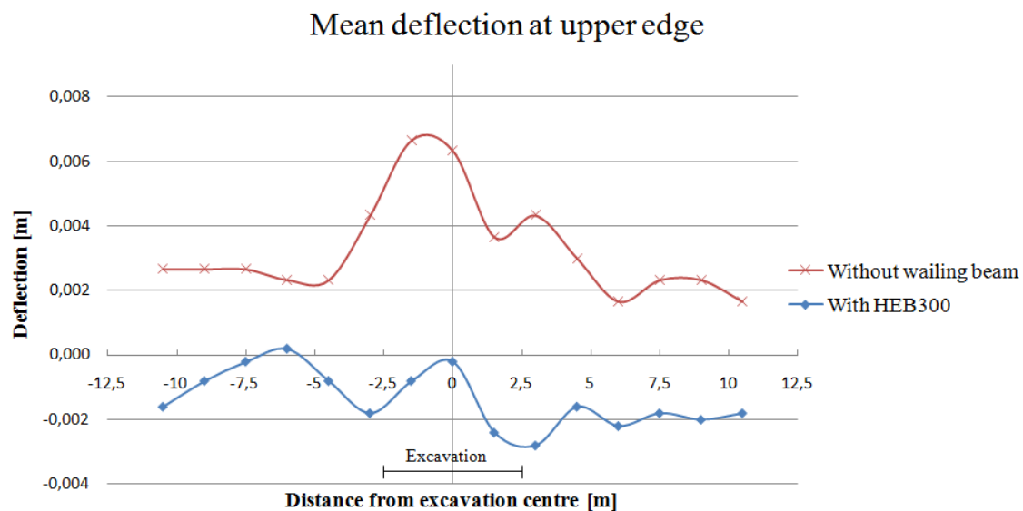
Figure 5.5 Mean values for the measured horizontal deflection at upper edge of the sheet pile wall for sections with and without wailing beam.
